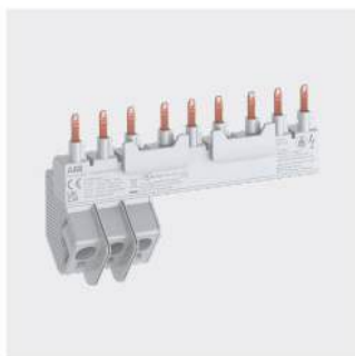
PS1-...-65K busbars for 2, 3, 4 or 5 manual motor starters
